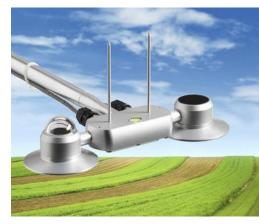
LP NET 14 is a 4-component Net-Radiometer for the measurement of the net radiation between  $0.3\mu$ m and  $45 \mu$ m. The net-radiometer consists of two pyranometers (one for the measurement of the global radiation and the other one for the measurement of the reflected solar radiation) and a pair of pyrgeometers (one for the measurement of the infrared radiation emitted by the sky and the other one for the infrared emitted by the ground surface).
